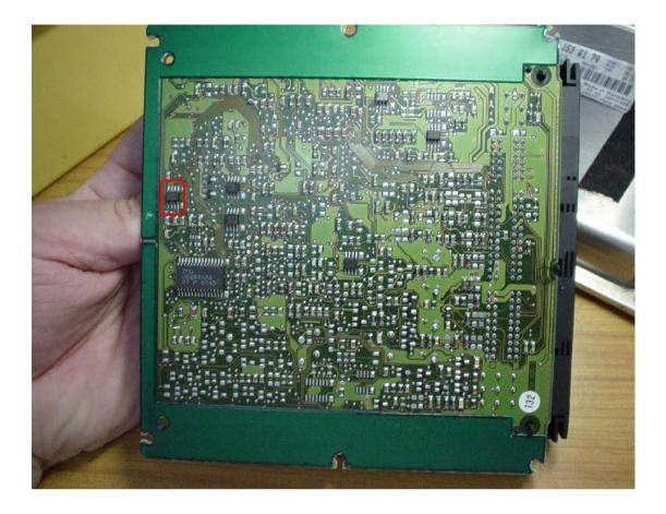
In the ECM of Sprinter, ML CR2 engine, 5 plugs, find memory 5P08C3 (read and type as SPI 95040).
